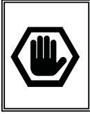
Emergency Stop Position
