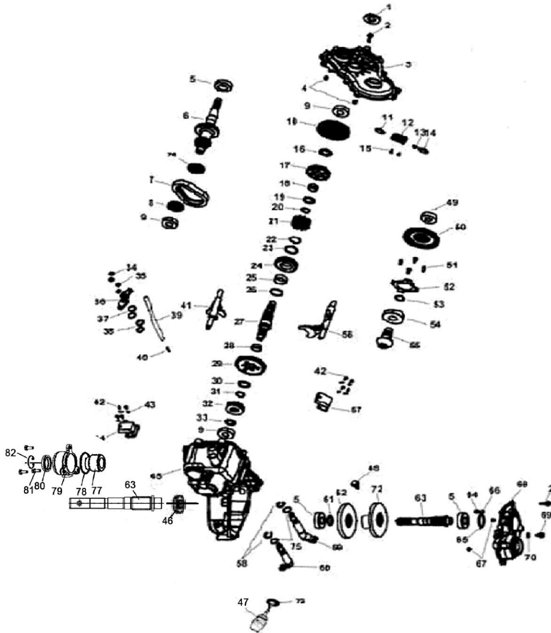
FIG 9: TRANSMISSION, 2WD / TRANSMISSION, 2WD
